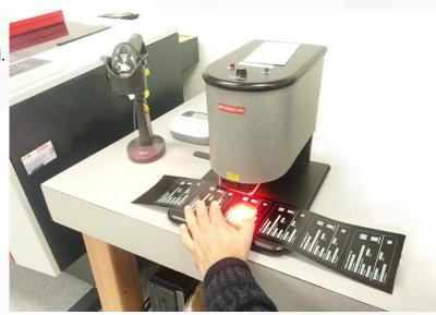
**IUID** verifier – for verifying the quality of the printed or etched barcode and whether the machine readable barcode conforms to MIL STD 130.
