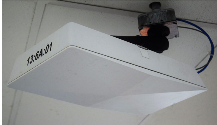
Fixed RFID readers from Impinj are used to detect products autonomously as they move between locations, updating the A2B Tracking asset dashboard with the latest date, time and location
