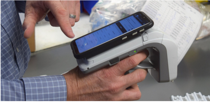
Using a smartphone to manage the RFID reader made training fast and simple for any user responsible for inventorying or locating products throughout the day
