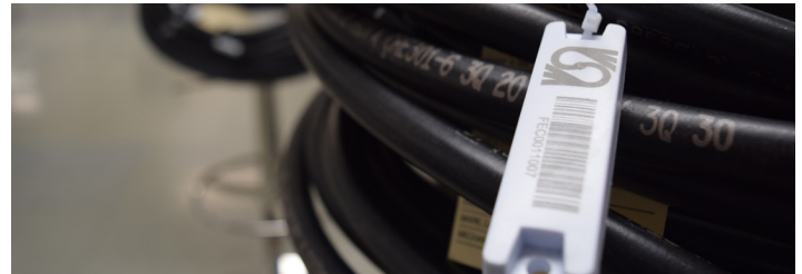
RFID tag selection was key to ensure that tags could be easily read when stacked on top of each other, or when placed within storage bins/totes and hidden from line of sight
